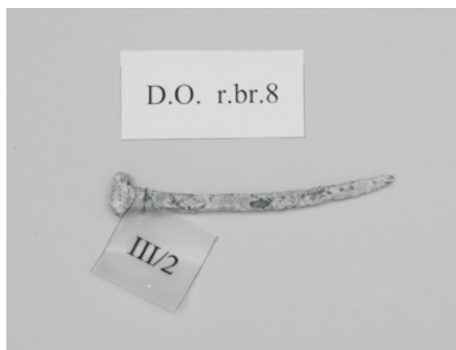
Fig. 27: Huge iron nail from the suspension bridge
