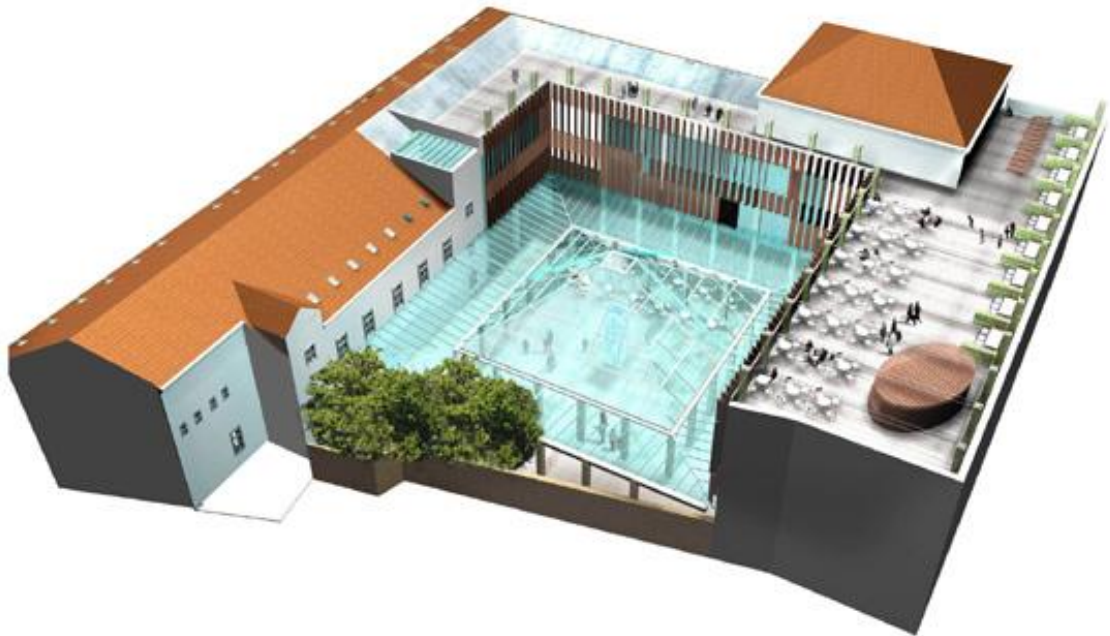
Bird's eye view of the core of the converted building with the added interior elevations and the glass roof of the new covered atrium
